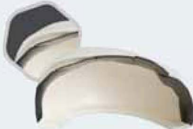
Traditional toe-protection and toe-cap gluing
